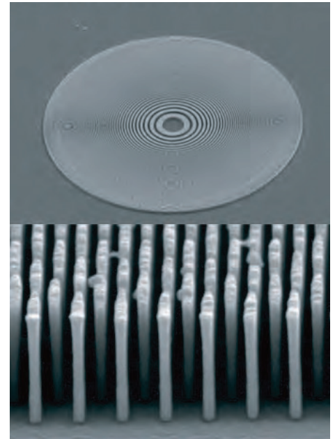
Figure: 1.1 Electroplated gold zone plate for multi-keV X-rays with 50 nm wide and 500 nm high structures
