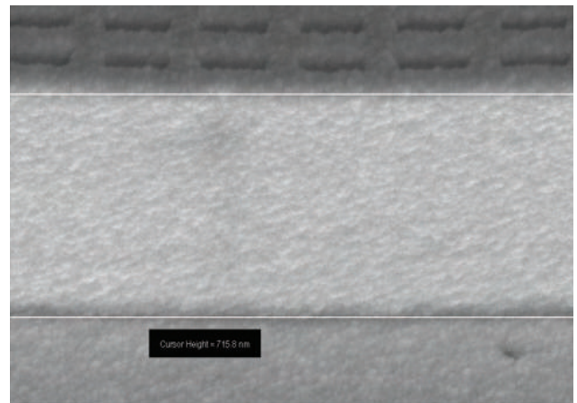
figure: 7.4 Tilted view (30°) of the zone plate with a height of 1430 nm. Due to geometric distortion, the actual height is twice the measured height
